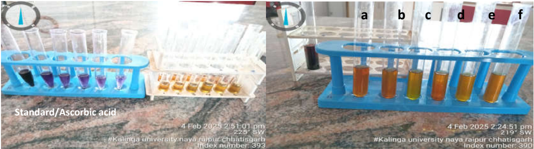
Fig(a) Fig(b) Fig1.4(a) Standard /ascorbic acid Showing DPPH assay (b) Showing DPPH assayfor different samples,where a,b,c are leaves of B.alba , P.oleracea , C. benghalensis and c,d,e are microgreens.
