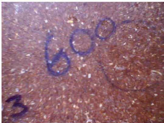
Figure9 600µm Grain size composite model
