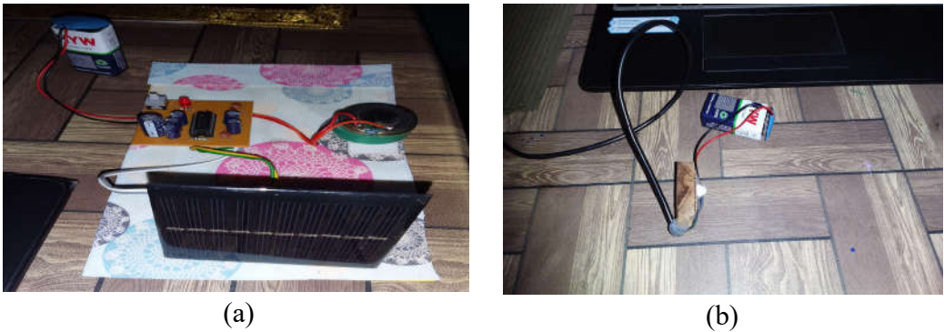
Figure 3 Hardware circuit of Li-Fi a) Receiver b) Transmitter
