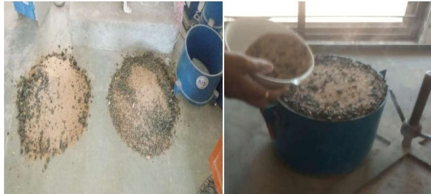
**Figure 1 Test procedures to calculate experimental packing density**
