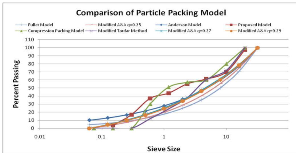
**Figure 3 Comparison of PPM based on PSD Curve**
